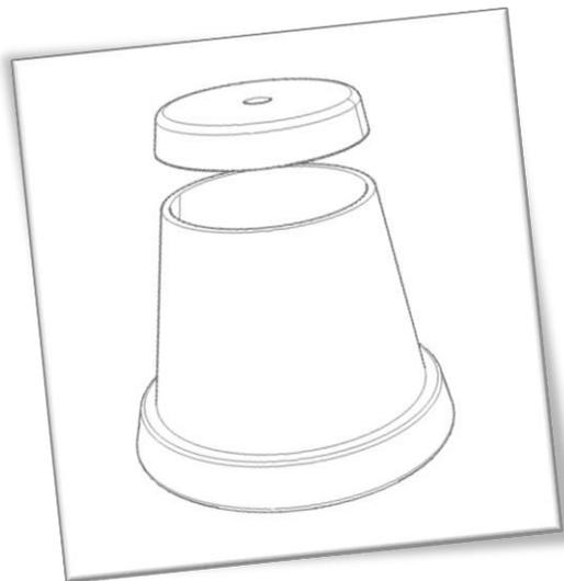
**Step 3:** Turn your plant pot bottom side up, and measure about 3cm. Use your angle grinder, with a masonry cutting disk fitted, to cut away the top, save it as you will need this later to cover your oven.
